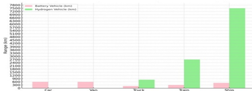
Fig.2. Comparison of battery electric and hydrogen vehicle range by transport mode
